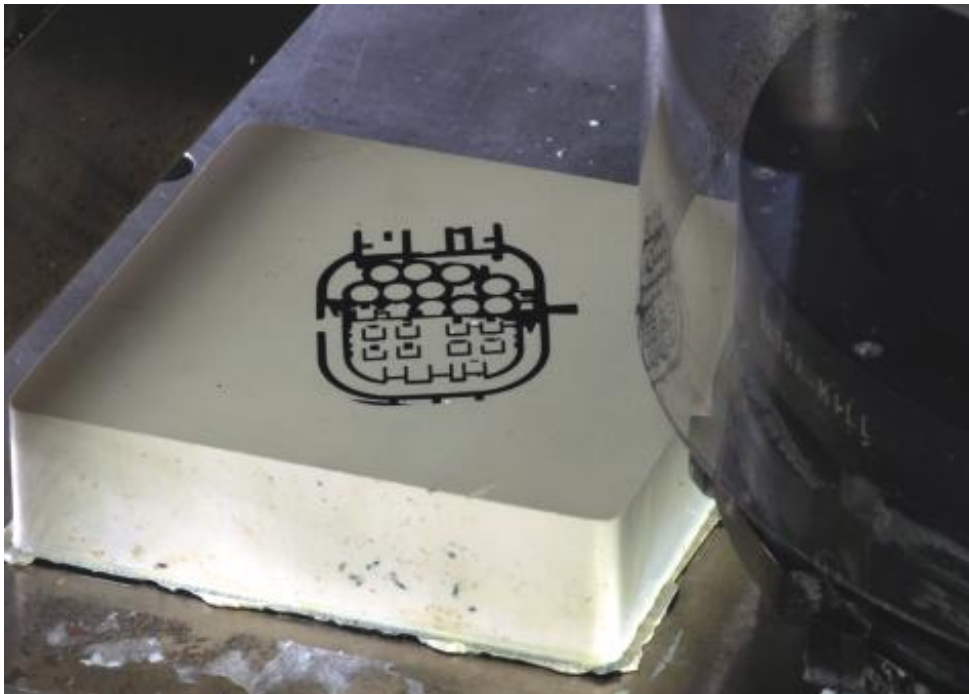
Above: This electrical socket is the same part as in the picture to the left. This shows CSS's ability to scan complex, inaccessible features.
